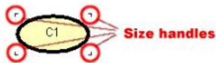
Figure 1: The size handles are placed at the four “corners” of the node
